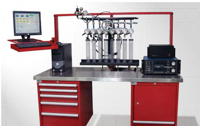
The FAST™ R&D Fuel Flow Bench is a custom built fuel injector dyno that is unequaled. Designed by FAST™ engineers, the one-of-a-kind system allows for advanced testing and development of an injector's flow capabilities.
